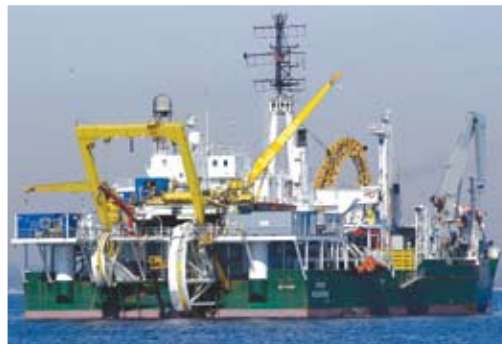
The Nexans Skagerrak is heading back to Norway after installing more than 30 miles of new 138-kV transmission cable between Norwalk, Conn., and Northport, N.Y., in February. The ship and her crew worked around the clock to install, bury and survey three 11-mile cable lengths. The new cables replace seven original cables installed nearly 40 years ago.
